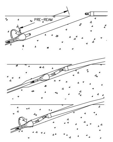
*Step 1* Pre-ream hole to minimum of one drill rod length.
