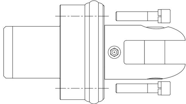
4. To remove the swivel, remove the six socket head capscrews. Use the jacking screws to break the joint between the flange and the reamer.
