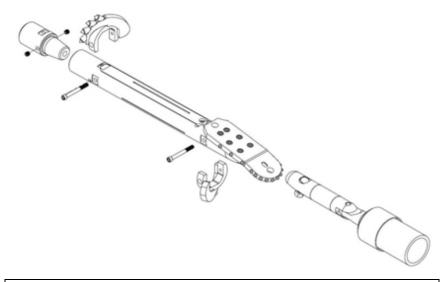
Melfred Borzall's Patent-Pending FastBack System is the quickest and easiest way to get product pulled and the job finished. Now the same housing, tailpiece and bit used on the pilot bore can be converted in to a reaming tool for soft short shots in soft ground.
