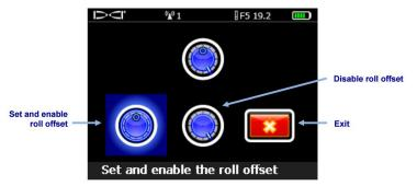
2. Ensure the drill head is at its 12 o'clock position and that the transmitter is on. Note the roll value showing on the screen.
