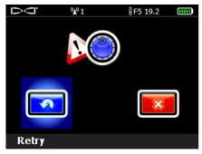
Click the trigger to retry setting the roll offset or toggle right to select exit and return to the setting menu. If the roll offset failure screen appears, verify the setup and try again or contact DCI Customer Service.
