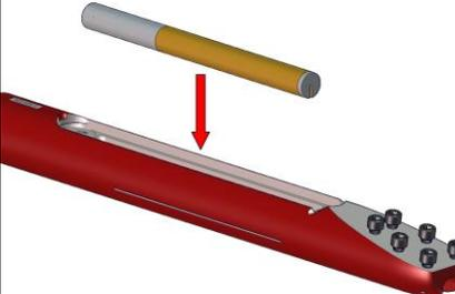
A diagram showing a yellow and grey transmitter being inserted into a pocket on the red cylindrical tool. A red arrow points down to the transmitter's position.                                                                                             |
