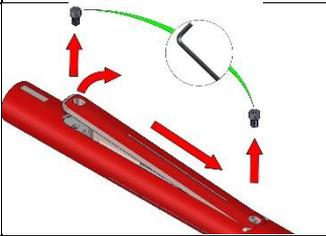
A diagram of a red cylindrical lid with two bolts. Red arrows indicate the lid being slid forward and then prying up from the back. A circular inset shows a hex key being used to remove a bolt. |
