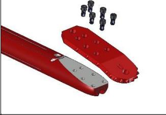
A diagram showing a red directional blade being attached to a red housing. Several bolts are shown above the blade, and a red arrow points to the blade's position.                              |
