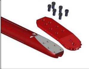
A diagram showing a red directional blade being attached to the housing. Several bolts are shown being inserted into the blade and tightened onto the housing.                                                                                                                |
