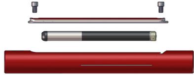
Melfred Borzall housings are built to last. They are machined from high quality, 4340 alloy steel and feature contoured pockets to eliminate stress concentrations, reducing the risk of cracking. Our unique lid design allows for larger locking bolts, keeping your investment safe in tough conditions. We've also made our housings easy to use by engraving the direction of drilling and the part number for easy identification. Here at Melfred Borzall, we've thought of everything; so you don't have to.
