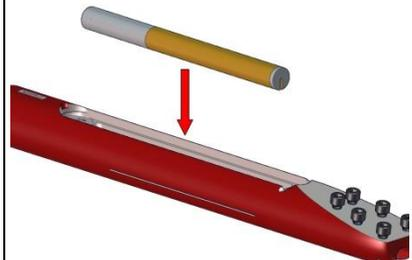
A diagram showing a yellow and white transmitter being inserted into a red housing. A red arrow points down to the transmitter being seated in the housing pocket.                                                                                                                            |
