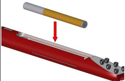
A yellow and grey transmitter is shown above a red housing. A red arrow points down to the mating tab in the housing pocket where the transmitter will be seated.                                                                              |
