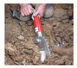
Key-way & bolt feature exclusive to Borzall Blades, ensures the swivel stays with the centerline rotation of the drill head
