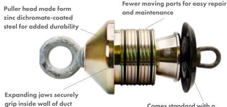
Comes standard with a polyurethane plugger to minimize fluid from entering the duct
