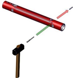
2. Remove the lid bolts. Then remove the lid by sliding it forward and prying up from the back.
