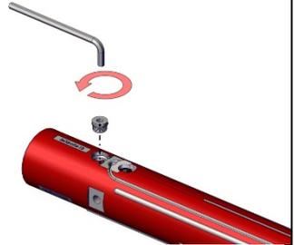
3. Install Item 12 (NOZ-0.25-0.75-16) by screwing into the port using the 5/16" Allen wrench.
